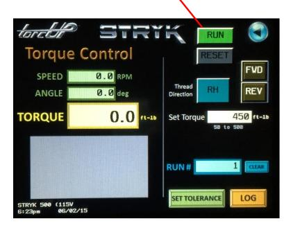
Each time the tool is operated, the indicator will flash either PASS or FAIL on the readout section of the control screen. The LED indicator on the rear of the tool handle will also show an indication of pass or fail, giving the operator a visual indicator without having to examine the control box.
