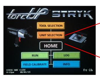
By pressing the UNIT SELECTION button, the screen to the right will appear. Operations for this mode are found detailed in the "UNIT SELECTION" Section.
